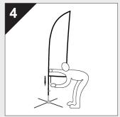
Slip on the waterbag onto the base, and then insert the pole. You can adjust the anchor point by moving it up or down to tighten or loosen the banner.
